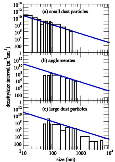
Fig1: Size distribution of dust particles collected using the vacuum collection. The solid line shows the Junge distribution.
