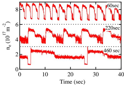
Fig. 2. Density response on gas puffing in a long duration discharge. The elapsed time from the beginning of the discharge shows in each sub-figure.
