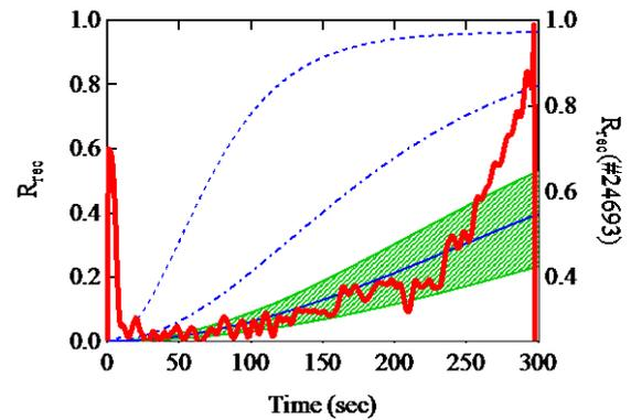
Fig. 3. Time evolutions of  $R_{rec}$  are calculated based on the QUEST-wall model. The solid, dotted, and dashed-dotted lines correspond to the cases of 100, 50, and 20 nm at H flux =  $2 \times 10^{17}$  H/m<sup>2</sup>/s. The hatched area shows the region of H flux from  $1$  to  $3 \times 10^{17}$  H/m<sup>2</sup> in the case of 100 nm. The thick solid line show the experimental result.
