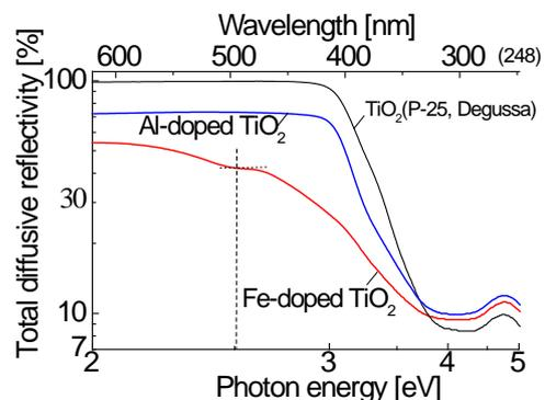
Fig.3 Total diffusive reflectivity of synthesized nanopowder.
