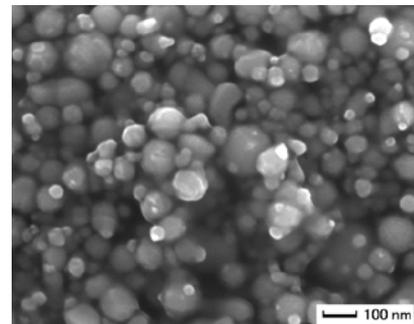
Fig. 2 FE-SEM images of synthesized Al-doped TiO<sub>2</sub> nanopowder.
