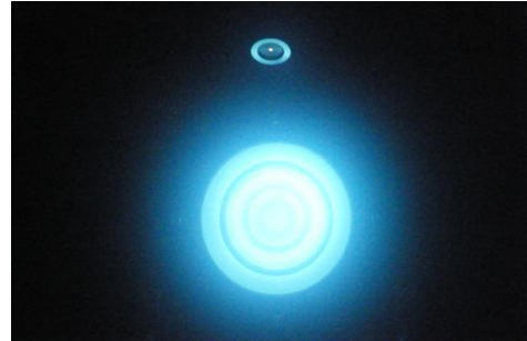
Fig. 3 High power xenon hall thruster operation in vacuum chamber in ISAS/JAXA.
