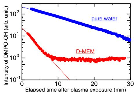
Fig.2. Temporal behavior of signal intensity of DMPO-OH adduct.
