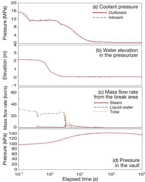
Fig. 2. Thermohydraulic transient behavior to the ex- VV LOCA.
