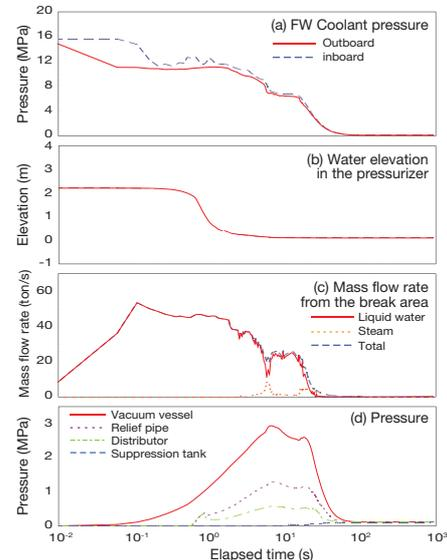
Fig. 3. Thermohydraulic transient behavior to the in- VV LOCA.
