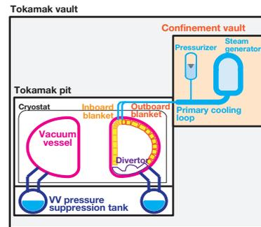
Fig.1. A schematic of the DEMO reactor analyzed.
