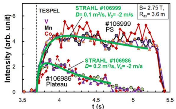
Fig. 1. Temporal evolutions of the  $K\alpha$  emissions of the tracers deposited directly inside the plasma in the cases of the PS and plateau regimes [2]
