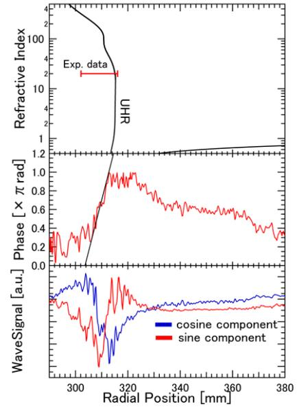
Fig.3. Comparison between refractive index profile and location for excitation of short wavelength mode.
