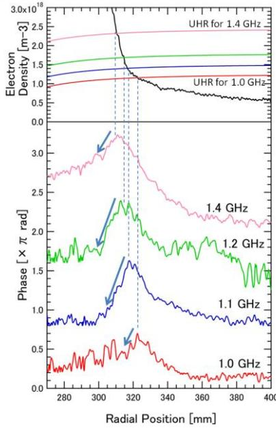
Fig.2. Phase profiles of electrostatic component (longitudinal wave mode) for several frequencies.
