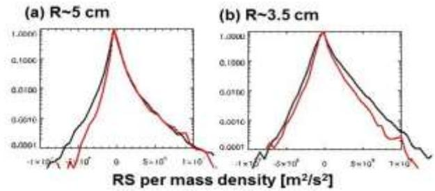
Fig.3. Results of conditional technique. Probability density functions of local Reynolds stress measured at (a)  $r = 5$  cm and (b)  $r = 3.5$  cm. Red and black plots indicate PDF in high state and low state, respectively.
