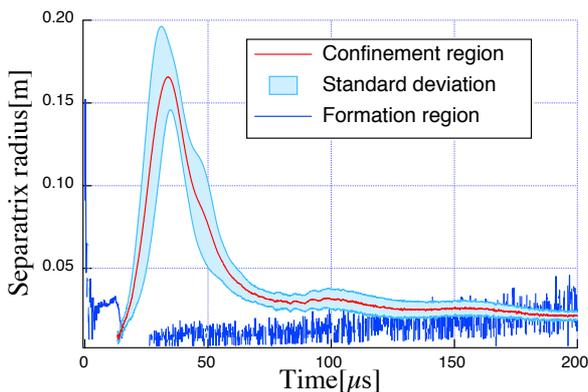
Fig.3. Time evolution of separatrix radius of FRC translated into a deuterium gas.
