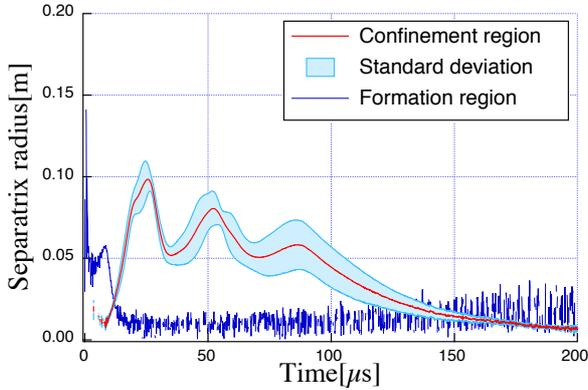
Fig.2. Time evolution of separatrix radius of a FRC translated into a vacuum confinement region
