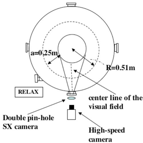
Fig.1 Top view of two-color imaging system.
