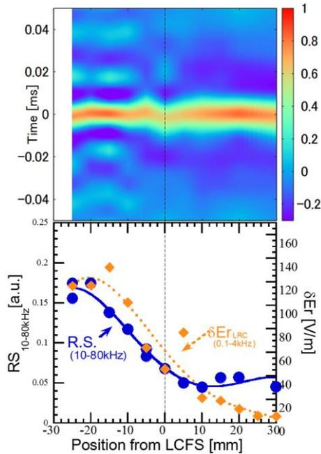
Fig. 2 (a) Cross-correlation between  $\delta E_r$  and  $\delta E_\theta$  in the frequency range of 10 to 80 kHz. (b) Reynolds stress calculated from the in the same frequency range.  $\delta E_{LCR}$  is also shown in the same figure for comparison.
