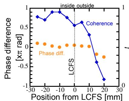
Fig. 1 Radial profile of phase difference and coherence  $\gamma$  at the frequency of 1 kHz between floating potential signals measured with a fixed probe and scanned probe around LCFS.
