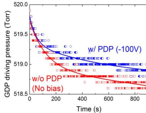
Fig.3 Variation of hydrogen gas pressures measured by an absolute pressure gauge at the gas side.
