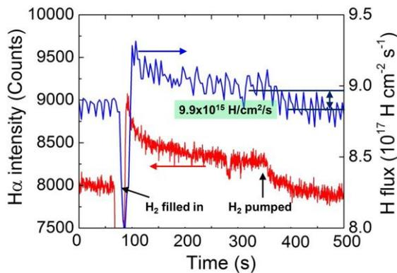
Fig.2 Hydrogen flux and H<sub>α</sub> signals detected in the upstream hydrogen plasma in VEHICLE-1.
