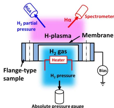
Fig.1 A schematic diagram of the bi-directional permeation setup in VEHICLE-1.
