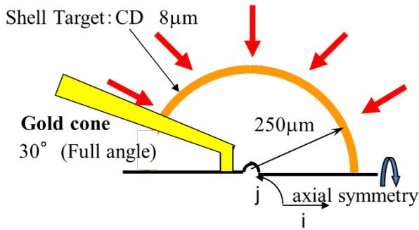
Fig.1. Initial conditions of the simulation. (a) CD shell target with inserted gold cone target and (b) uniform initial magnetic field of which intensity is 300T
