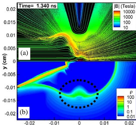
Fig.2. Snapshots of (a) magnetic field lines (colors in Tesla), and (b) mass density ( $\text{g}/\text{cm}^3$ ) at an acceleration phase (1.34 ns). The magnetic field is compressed along with the mass compression. In the dotted circle, a mass perturbation is seeded at early phase due to the electron heat flux limitation for the strong magnetic field.
