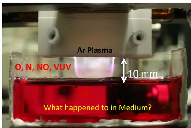
Fig. 2. The photograph of plasma treatment of medium. The atmospheric pressure Ar plasma was exposed to the medium with a distance of 10mm.
