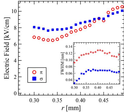
Fig.2. Electric field distribution derived by the analysis of the Stark splitting on each polarization. Inset shows line width fitted for each Stark-split transition component.
