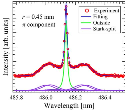
Fig.1. Stark-split  $H_{\beta}$  spectrum of  $\pi$  polarization component, curve reproduced by using theoretical relative intensities, and each component obtained by fitting procedure [ $r=0.45$  mm].
