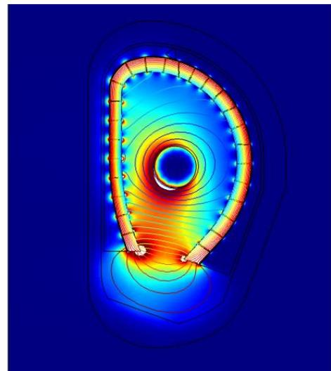
Fig. 3. Magnetic flux surfaces and color map of magnetic flux density ( $f = 1\text{Hz}, \mu_r = 1000$ )
