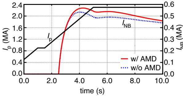
Fig. 1. Time evolution of the NB driven current
