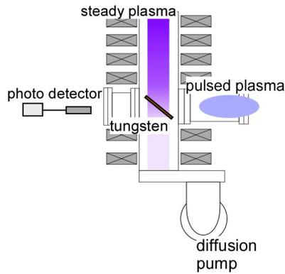
Figure 1. Schematic of the experimental device, NAGDIS-PG.
