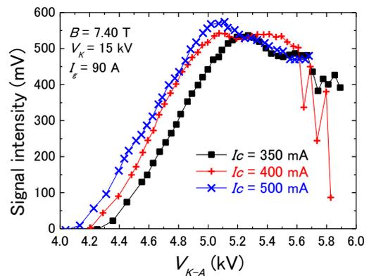
Fig 2. Measured signal intensity with changing  $V_{K-A}$
