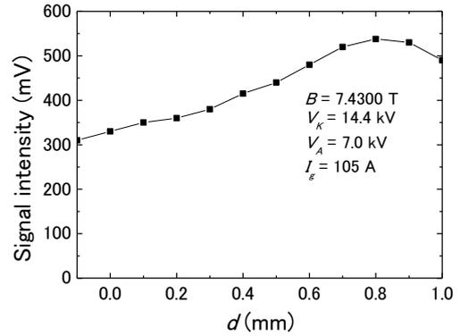
Fig 1. Measured signal intensity with changing the gyrotron tube position
