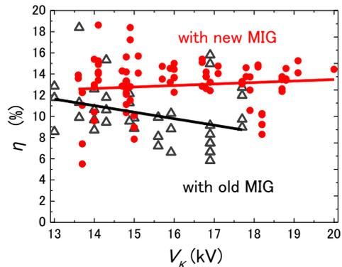
Fig 3. The efficiency  $\eta$  obtained by the power measurement with the new MIG (red circles) and with the old one (black triangles)
