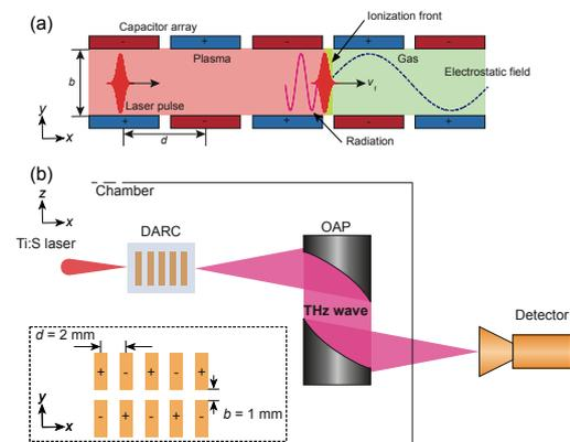
Fig. 1. (a) Schematic of the DARC. (b) Schematic of the experimental setup.
