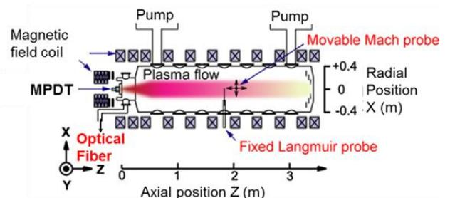
Fig.1. Schematic of HITOP device
