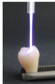
Fig. 2. LF jet irradiation on the caries tooth model
