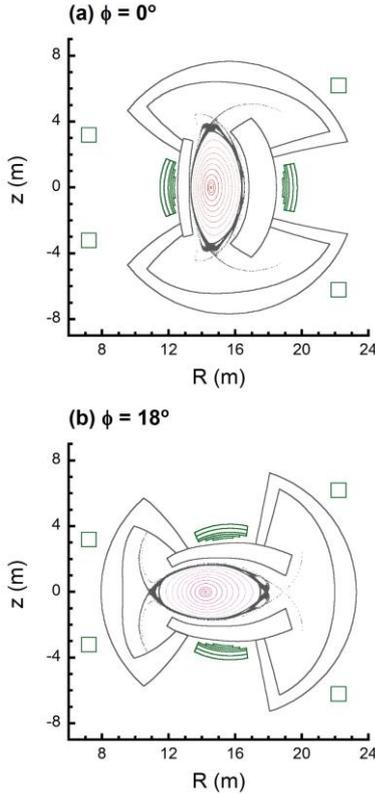
Fig.1. Vacuum magnetic surfaces of FFHR-d1A at toroidal angles (a)  $\phi = 0^\circ$  and (b)  $18^\circ$ .
