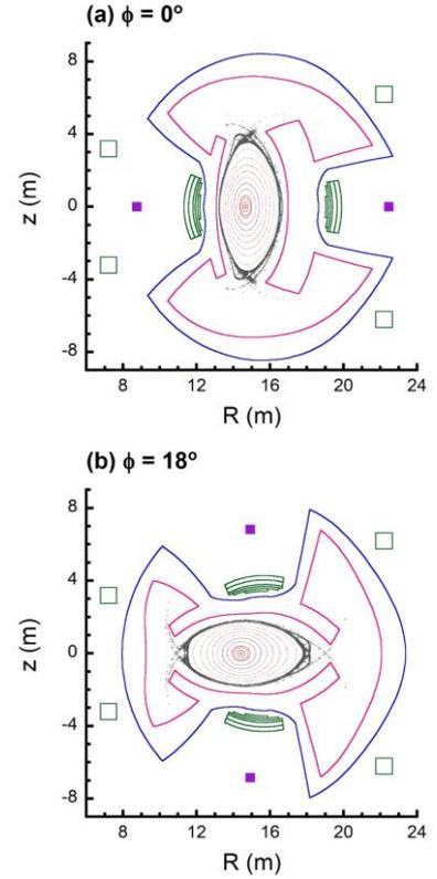
Fig.3. Vacuum magnetic surfaces of FFHR-d1C-TW at toroidal angles (a)  $\phi = 0^\circ$  and (b)  $18^\circ$ .
