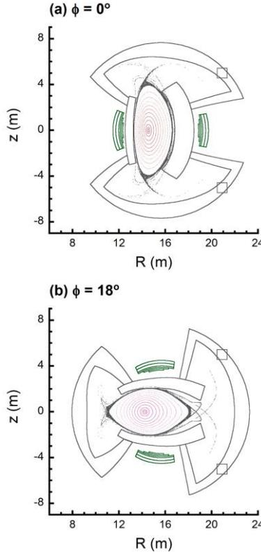
Fig.2. Vacuum magnetic surfaces of FFHR-d1C-BE at toroidal angles (a)  $\phi = 0^\circ$  and (b)  $18^\circ$ .
