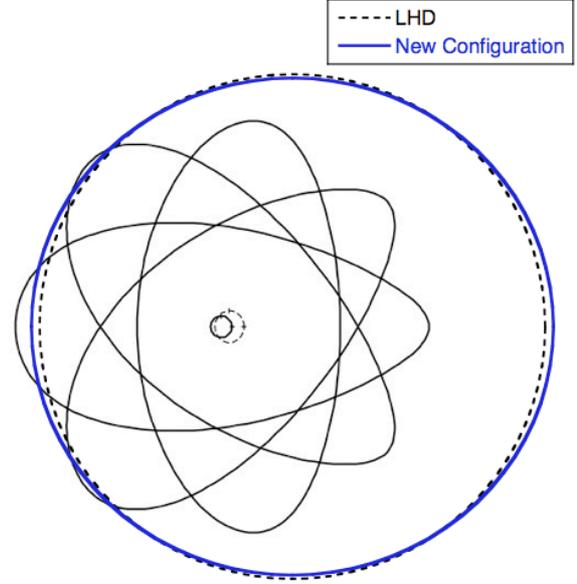
Fig. 2 Cross section of helical coil winding surfaces of LHD-SS1 and LHD. Four cross sections of boundary surface of LHD-SS1 are also shown.
