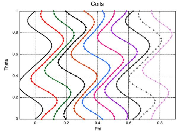
Fig. 3 Coil filament traces of modular coils on the winding surface. 10 modular coils are designed for one toroidal period of LHD-SS1.
