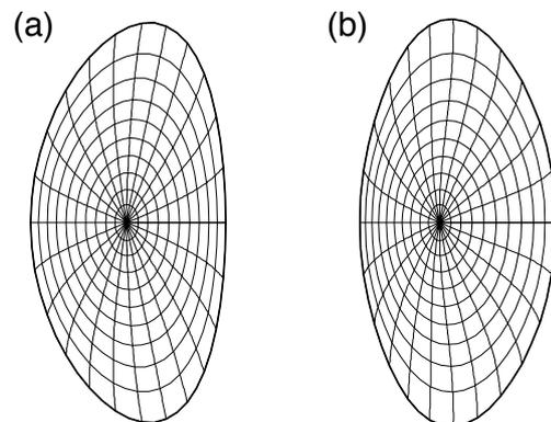
Fig. 1 Comparison of boundary shapes of vertically elongated cross section of (a) LHD-SS1 and (b) LHD inward shifted configuration.
