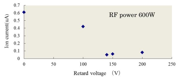
Fig.3. Retard ion current measurement. The N<sub>2</sub> flow rate is 10 sccm. The measuring position is 100 mm in the downstream from the flux exit.
