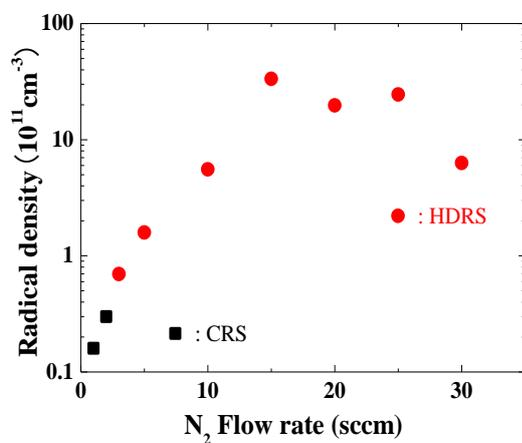
Fig.2. Absolute density of nitrogen radicals as a function of the flow rate.
