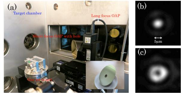
Fig. 4. (a) Focusing system. (b) Laser spot pattern of linearly polarized pulse. (c) Radially polarized laser pulse
