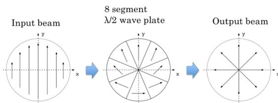
Fig. 3. Production of radially polarized laser pulse.
