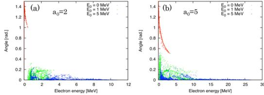
Fig. 1. Simulation results of laser normalized vector potential of the laser pulse at (a)  $a_0=2$  and (b)  $a_0=5$ . Initial electron kinetic energy is 0 MeV (red dots), 1 MeV (green dots), and 5 MeV (blue dots), respectively.
