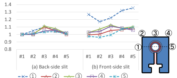
Fig. 4. Result of infrared thermography inspection
