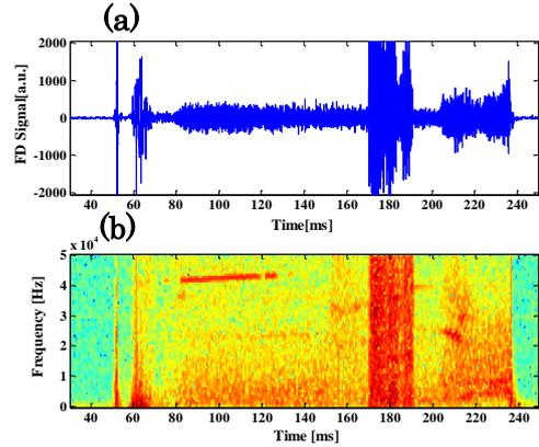
Fig.3 Time evolution of the FD raw signal (a) and the FFT spectrogram (b) of channel 4.
