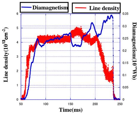
Fig.2 Electron density and diamagnetism.
