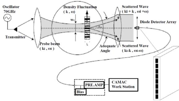
Fig. 1. Schematic diagram of FD method system.
