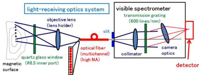
Fig.2. Schematic of the visible spectrometer system
