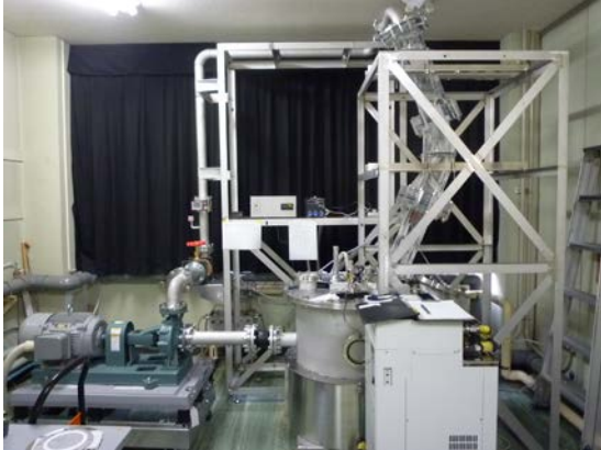
Fig.3. Over view of the experimental water flowing device.
