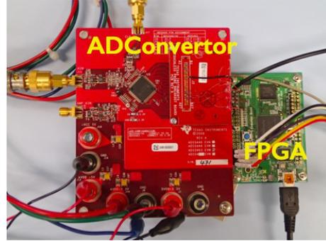
Fig. 2: Picture of the HYADC prototype using evaluation boards.
