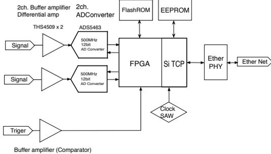
Fig. 1: Circuit diagram of The HYADC.
