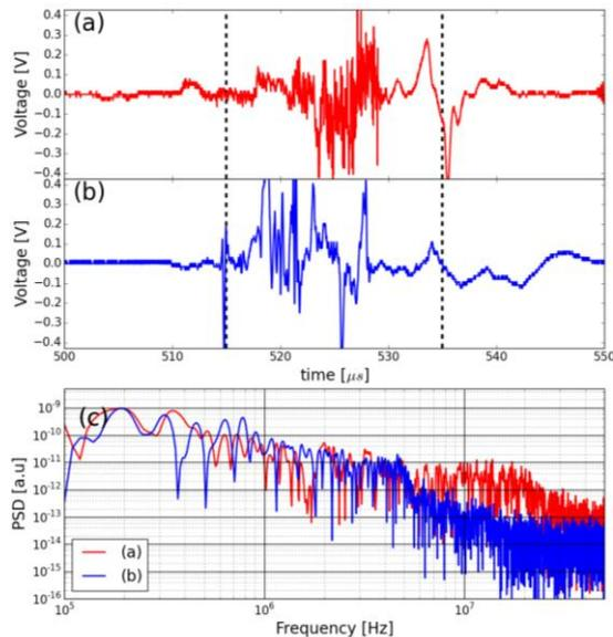
Fig. 2. (a), (b) Magnetic fluctuation signals measured by L-shaped magnetic fluctuation probe in counter-helicity merging experiment and (c) power spectral density (PSD) of fluctuation signals in (a) (red) and (b) (blue). The fluctuation signals between dotted lines in (a) and (b) were used to calculate PSD (515-535 μs)
