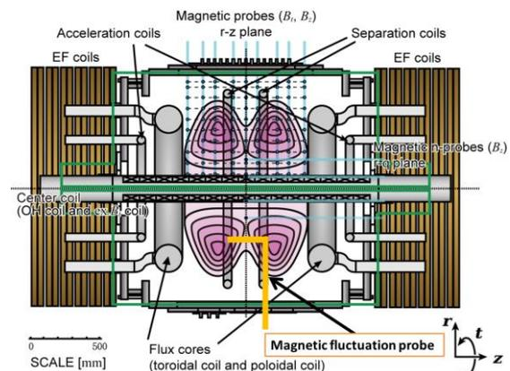
Fig. 1. An overview of plasma merging device TS-4 and experimental setup of magnetic fluctuation probe.
