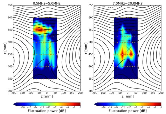
Fig. 3. The fluctuation power distribution of (left) 0.5-5 MHz and (right) 7-20 MHz frequency range measured by L-shaped magnetic fluctuation probe and poloidal magnetic flux contour (black line) measured by 2-D magnetic probe. Orange dots indicate measurement points and black x-mark denotes the X-point.
