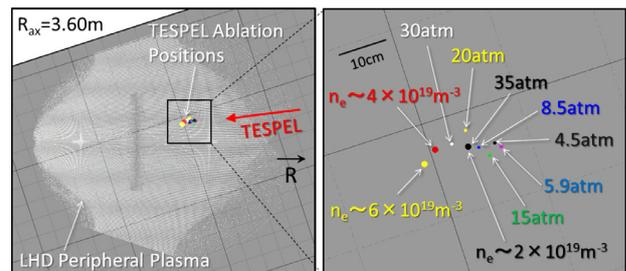
Fig.1. Top view of a LHD peripheral plasma with indication of the three-dimensional ablation positions of the encapsulated impurity (tungsten) injected by the TESPEL when the propellant gas pressure and the plasma density were changed.
