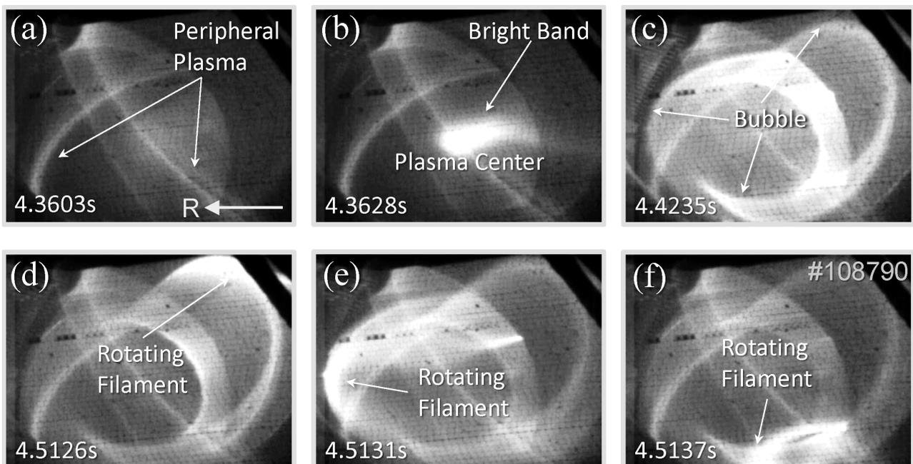
Fig.2. Sequential images of a tangential view of an LHD plasma observed with a fast-framing camera after tungsten encapsulated pellet injection. A self-organized rotating filament structure appeared around the core plasma.
