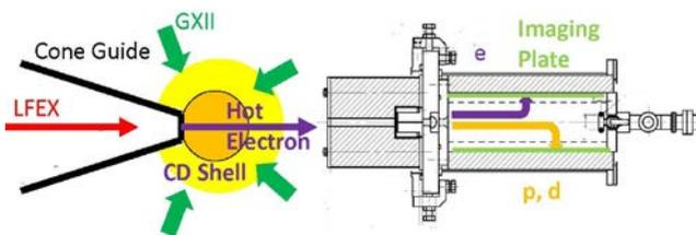
Fig. 1 The experimental setup and Electron/Ion Spectrometer.
