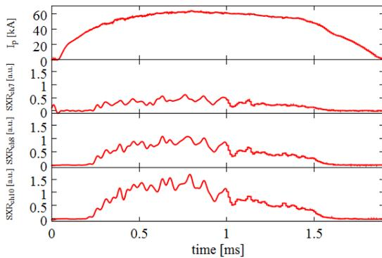
Fig.2. Time evolution of the toroidal plasma current and SXR emission signals.
