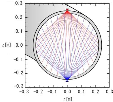
Fig.1. Ploidal cross-section of RELAX with lines of sight of each photodiode
