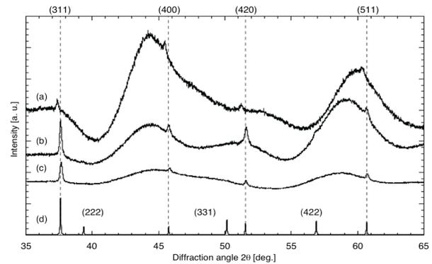
**Fig. 3.** The X-ray diffraction one-dimensional profile from the YSZ. (a) Irradiated with ns-Beam. (b) Irradiated with ps-Beam. (c) Irradiated with fs-Beam. (d) Non-irradiated YSZ.
