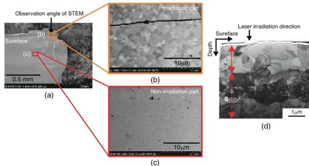
**Fig. 2.** (a) SEM image on the OAP1 side of irradiated with fs-Beam. (b) Enlarged view of reflection electron image at irradiation area with fs-Beam of (a). (c) Enlarged view of reflection electron image at non-irradiation area of (a). (d) Cross-sectional of irradiated part with fs-Beam observed by STEM: L is large crystal grain layer. S is small crystal grain layer
