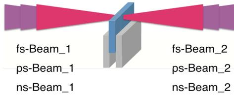
**Fig. 1. Irradiation layout on the YSZ**
