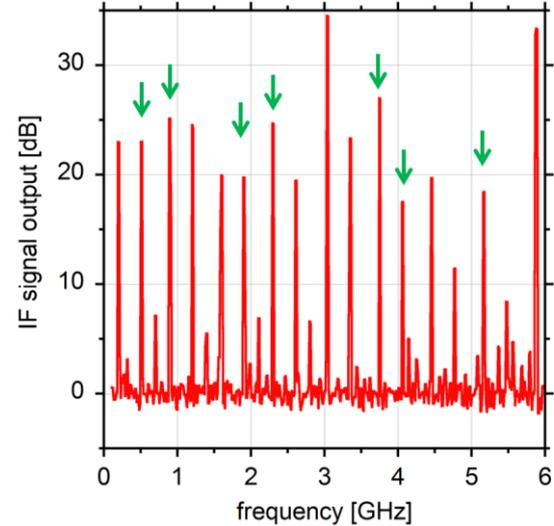
Fig.1. Frequency spectrum of the IF signal, which is the microwave mixer output. The arrows indicate the utilized frequency components in the filter bank system.
