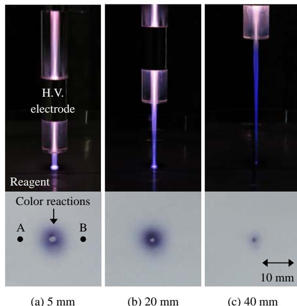
Fig. 2. Influence of the irradiation distance (a) 5 mm, (b) 20 mm and (c) 40 mm on the plasma jet and the resulting ROS distribution. Points A and B are used in Fig. 3.
