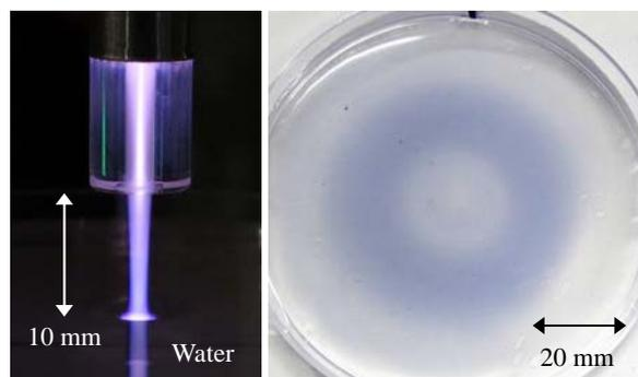
Fig. 4. Plasma jet irradiated to water and the resulting ROS distribution in the bottom of water. The irradiation distance and time were 10 mm and 60 min, respectively.
