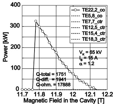
Fig.2. Calculated power of the TE<sub>22,2</sub> mode
