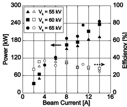
Fig.1. Measured power and efficiency
