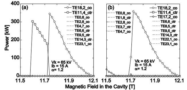
Fig.3. Result of mode competition calculation. Fig. (a) includes TE<sub>18,2</sub>, TE<sub>11,4</sub> and other near modes. Fig. (b) includes TE<sub>18,2</sub>, TE<sub>11,4</sub>, TE<sub>17,2</sub> and other near modes.
