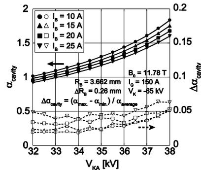
Fig.4. Plots of  $\alpha_{\text{cavity}}$  and  $\Delta\alpha_{\text{cavity}}$  as functions of  $I_B$  and  $V_{KA}$
