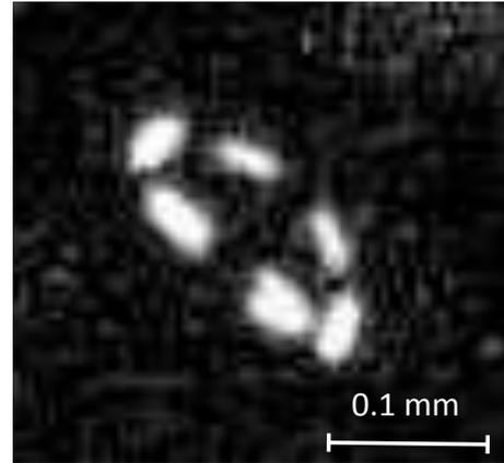
Fig. 5 An orbit of a SiC particle (side view). 10 images are superimposed.  $V_{RF} = 280 \text{ V}_{\text{rms}}$ ,  $I_{RF} = 0.2 \text{ A}_{\text{rms}}$ ,  $p(\text{Ar}) = 12 \text{ Pa}$ .
