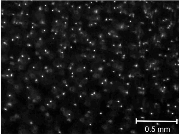
Fig. 3 Lattice-like 3D structure of  $\text{Si}_3\text{N}_4$  in the HF Plasma (side view).  $V_{RF} = 280 \text{ V}_{\text{rms}}$ ,  $I_{RF} = 0.2 \text{ A}_{\text{rms}}$ ,  $f = 100 \text{ kHz}$ ,  $p(\text{Ar}) = 13 \text{ Pa}$ .
