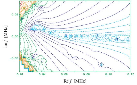
Fig. 5 Frequency spectrum with fast ion component,  $n_{F0} = 1 \times 10^{17} \text{ m}^{-3}$ ,  $T_{F0} = 0.5 \text{ MeV}$
