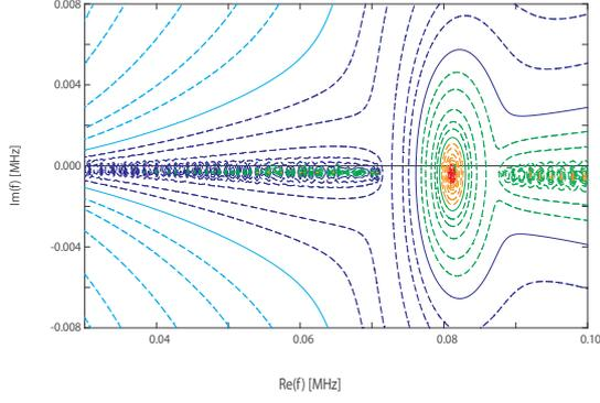
Fig. 2 Contour of  $|E|^2$  in complex frequency space with collisional cold plasma model
