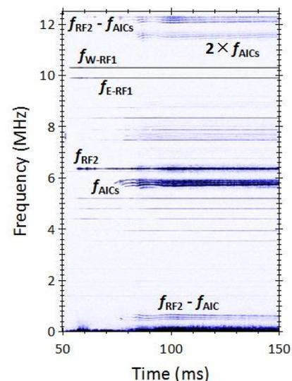
Fig. 1. Density fluctuation spectrum measured by a reflectometer in the GAMMA 10 central cell.
