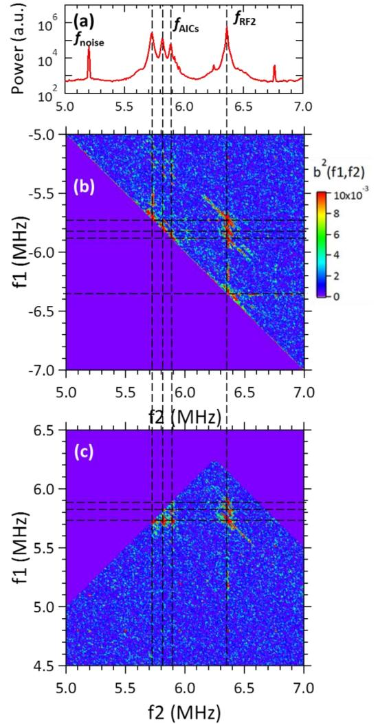
Fig. 2. (a) Ensemble averaged power spectrum of the density fluctuation measured by a reflectometer and (b), (c) its bicoherences.
