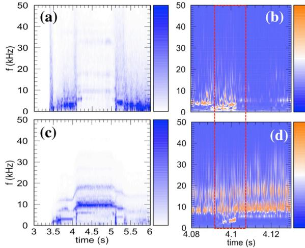
Fig.2. Temporal evolutions of (a) power and (b) wavelet spectrum of the density fluctuations at the edge plasma region ( $R \approx 4.6$  m), and (c) power and (d) wavelet spectrum of the magnetic fluctuations as a function of frequency.
