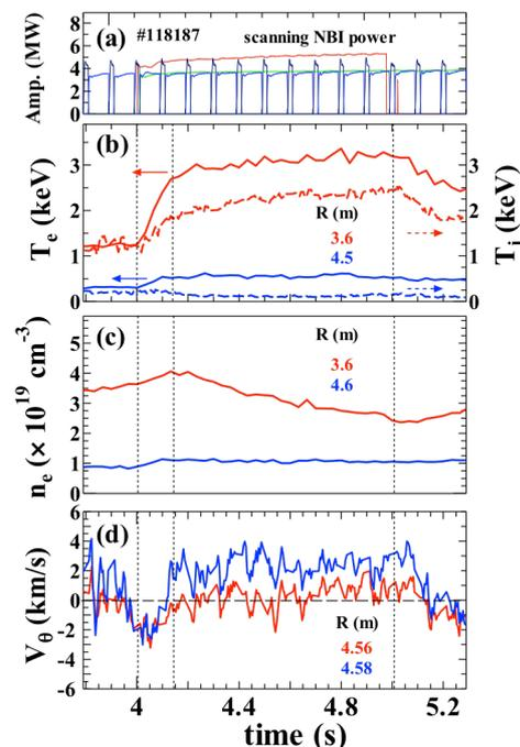
Fig. 1. Time evolution of (a) the NBI powers, (b) the electron temperature ( $T_e$ ) and ion temperatures ( $T_i$ ), (c) the electron density ( $n_e$ ), and (d) the poloidal rotation velocity ( $V_\theta$ ) in the LHD.
