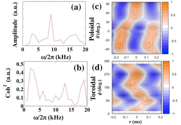
Fig.3. (a) Auto-power spectrum of magnetic fluctuations, and (b) cross-coherence spectrum between density and magnetic fluctuations, and contour plot of the cross-correlation function of the magnetic fluctuations with  $f \approx 2-5$  kHz for (c) poloidal and (d) toroidal directions at  $t \approx 4.1$  s.
