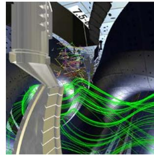
Fig.1. Integrated VR visualization of time-sequential data of dusts, equilibrium plasma simulation result and the inner surface of the LHD vacuum vessel. The dust trajectories are shown with the magnetic-field streamlines in green and red near the 7.5-U port.
