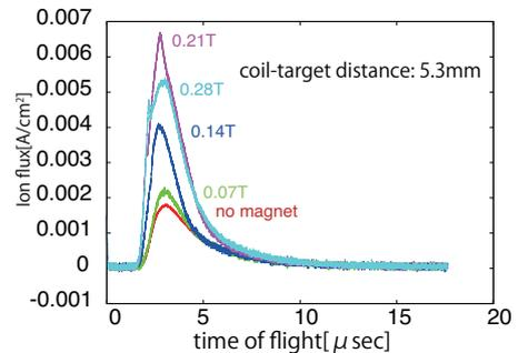
Fig.4. Plasma ion flux with changing field strength (measured at 170mm from the target).
