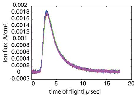
Fig.3. Ion flux waveforms (3 shots overlaid).
