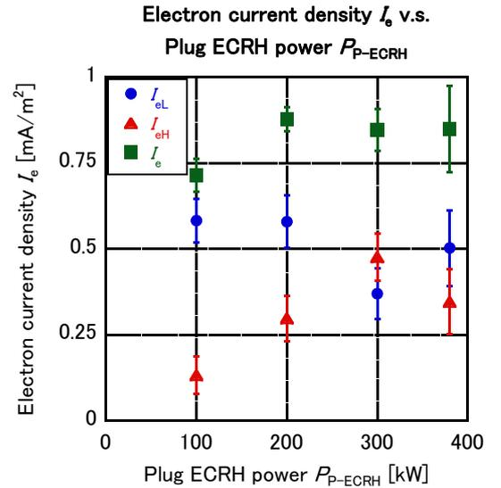
Fig. 3. The dependence of the electron current density on plug ECRH power in east LED
