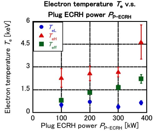
Fig. 2. The dependence of the electron temperature on plug ECRH power in east LED
