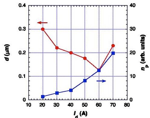
Fig. 5 Estimated cluster size & density vs. discharge current under normal gravity condition.  $p(\text{He})=40$  kPa,  $z=2$  cm.
