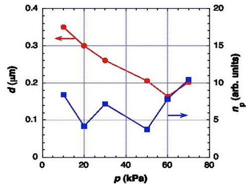
Fig. 4 Estimated cluster size & density vs. He pressure. Under normal gravity condition.  $I_d=40$  A,  $z=2$  cm.
