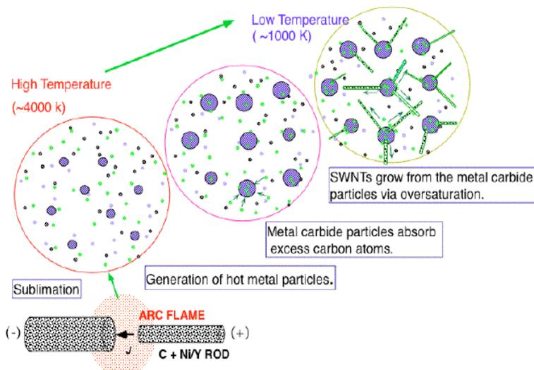
Fig. 1 A model figure of production process of CNTs by the arc discharge method.
