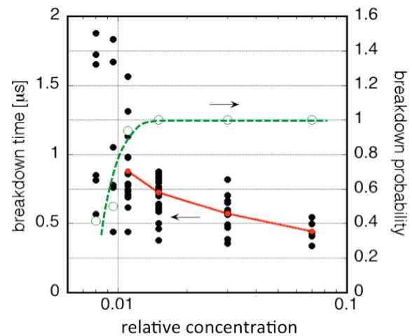
Fig.3. Statistics of the calculated discharge, showing the breakdown probability (open circle and green line), and breakdown time from each run (closed circle) and its averaged value (red line).
