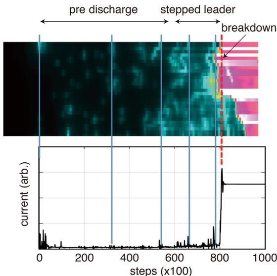
Fig.2. Simulated streak image from temporal and spatial evolution of the discharge and corresponding current at the upper electrode.
