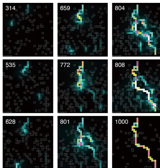
Fig.1. Profiles of current showing the development of a leader. The number in each figure corresponds to 1/100 of calculation steps. Open squares show the ionized cells, and the current is shown by the color.
