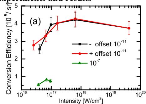
Fig. 1. The conversion efficiency as a function of laser contrast and intensity.
